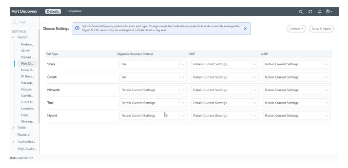
By default, GDP is enabled on the stack and circuit type ports. For the other port types, you can click the drop-down to either:
